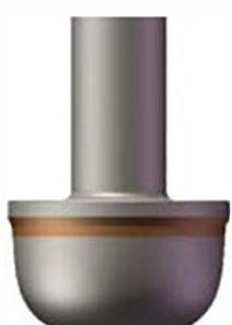
Partial welding on sealing face of plug
