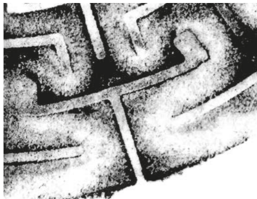
ACTUAL GASEOUS FLOW THROUGH RAVEN TRIM.
