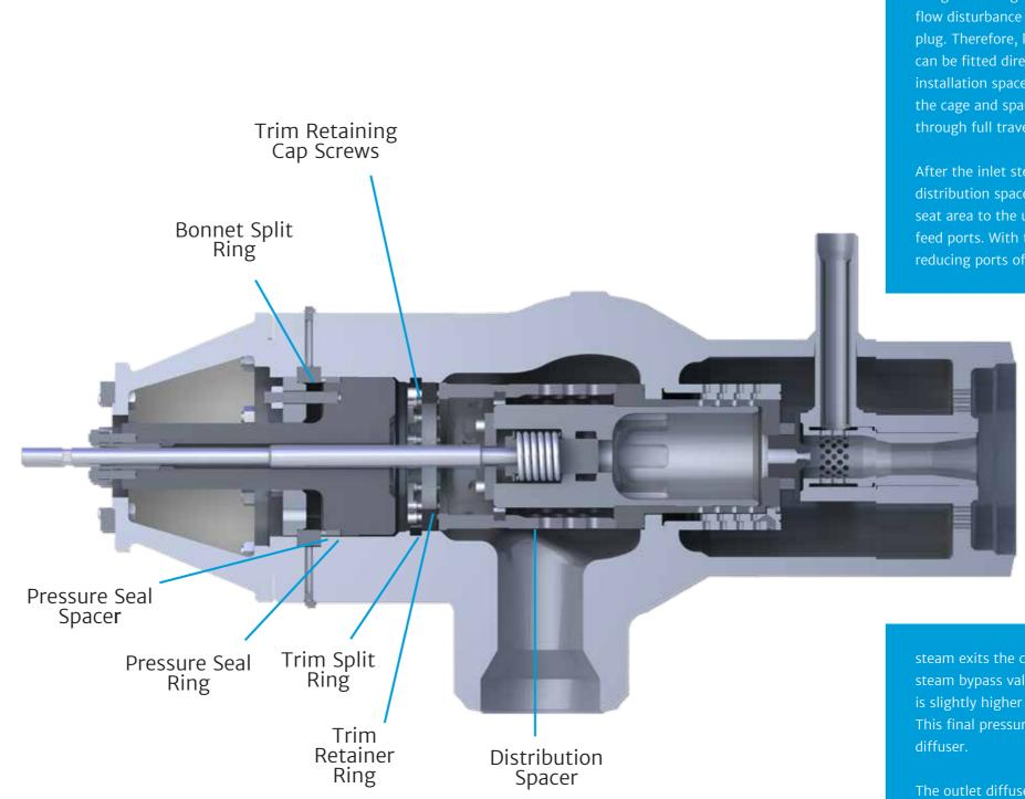
evenly positioned around the circumference. This heavy duty distribution spacer has been specifically designed to negate any upstream pipe work induced flow disturbance being communicated to the main plug. Therefore, long radius bends or isolation valves can be fitted directly to the valve inlet to minimize installation space. The main plug is fully guided by the cage and spacer to ensure complete plug stability through full travel.
