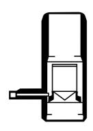
A VO-76 typically will be one nominal size smaller than the equivalent VO-II. Both will have the same size plug and internal components.
