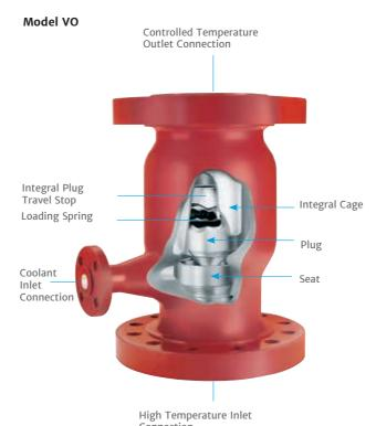
This pressure drop creates a relatively high velocity across the seat area, and it is at this point of low pressure constant velocity that the coolant is admitted into the vapor flow.
